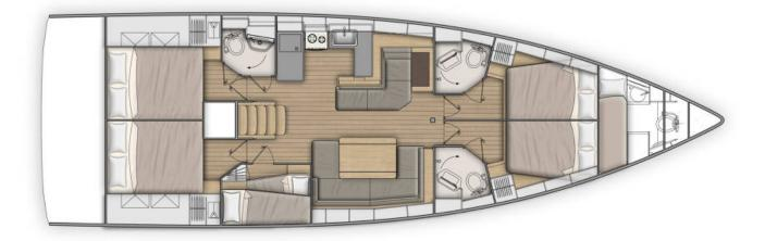
Shipyard: Beneteau Launched: 2018 Length overall: 15.94 m 14.98 m Length of the hull: Width 4.80 m Draft 1.92 m ca. 122 m<sup>2</sup> Sail Area: Mainsail halfsticked with lazy jack and lazy bag Furling genoa
