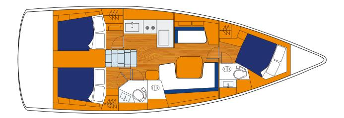
**Length Overall:** 12.43m/40ft 9in Waterline Length: 11.37m/37ft 4in 4.20m/13ft 9in Beam: **Draft:** 1.68m/5ft 6in **Displacement:** 7836kg/17271lb 200L/53gal **Fuel Capacity:** Water Capacity: 570L/150gal Yanmar 45hp **Engines:**
