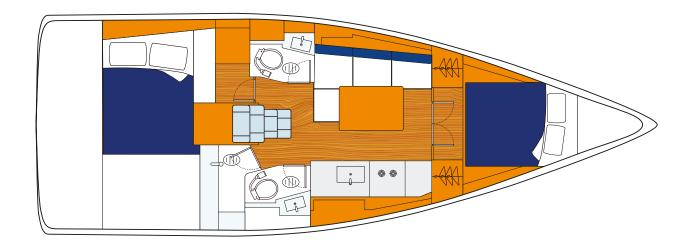
**Length Overall:** 11.50m/37ft 9in **Waterline Length:** 10.72m/35ft 2in 3.99m/13ft 1in Beam: 1.64m/5ft 5in **Draft: Displacement:** 15097kg/6850lb **Fuel Capacity:** 130L/34gal **Water Capacity:** 330L/87gal Yanmar 29hp Sail Drive **Engines:**
